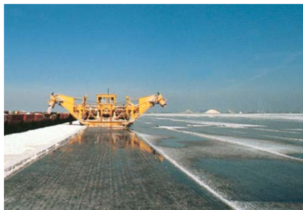
Solar evaporation process for obtaining sodium chloride.
