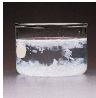
Precipitate formed by the reaction between \text{K}_3\text{PO}_4(\text{aq}) and \text{Ca}(\text{NO}_3)_2(\text{aq}) .
