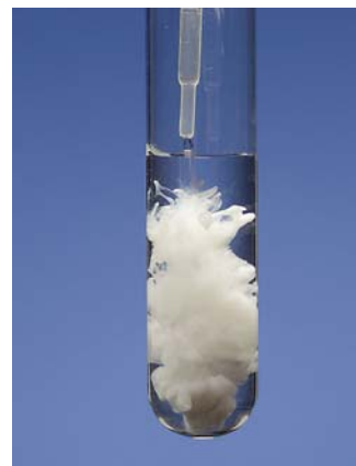
Figure 4.5 Formation of \text{BaSO}_4 precipitate.
