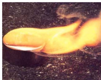
White phosphorus burns in air to form \text{P}_4\text{O}_{10} .
