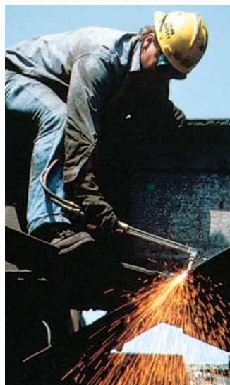
An oxyacetylene torch has a high flame temperature (3000°C) and is used to weld metals.
