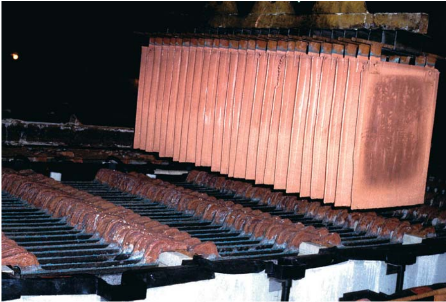
Figure 20.7 Copper cathodes used in the electrorefining process.
