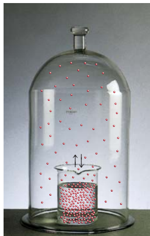
Liquid water in equilibrium with its vapor in a closed system at room temperature.
