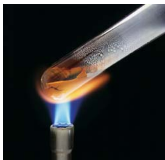
On heating, HgO decomposes to give Hg and O 2 .
