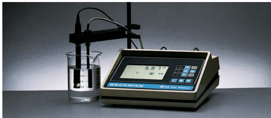
Figure 15.2 A pH meter is commonly used in the laboratory to determine the pH of a solution. Although many pH meters have scales marked with values from 1 to 14, pH values can, in fact, be less than 1 and greater than 14.
