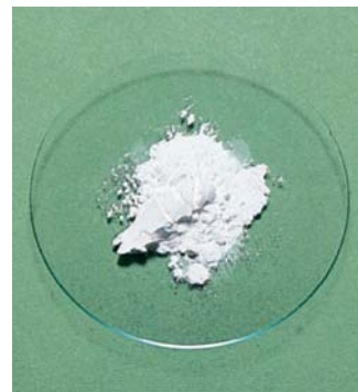
Lithium fluoride. Industrially, LiF (like most other ionic compounds) is obtained by purifying minerals containing the compound.
