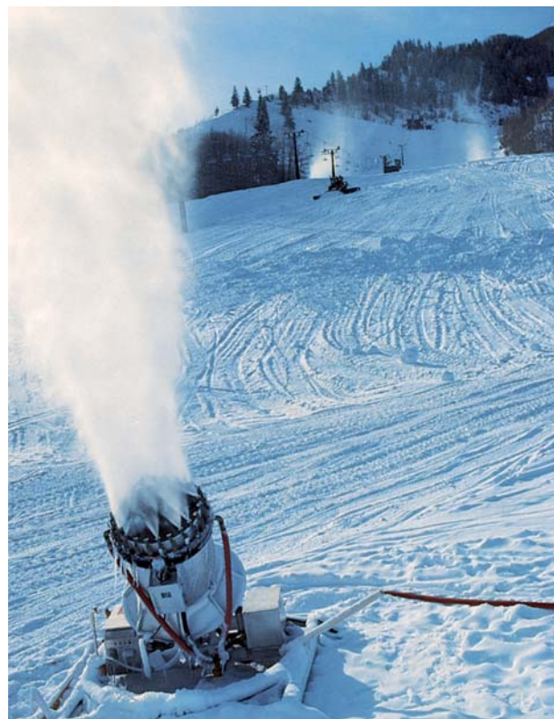
A snowmaking machine in operation.
