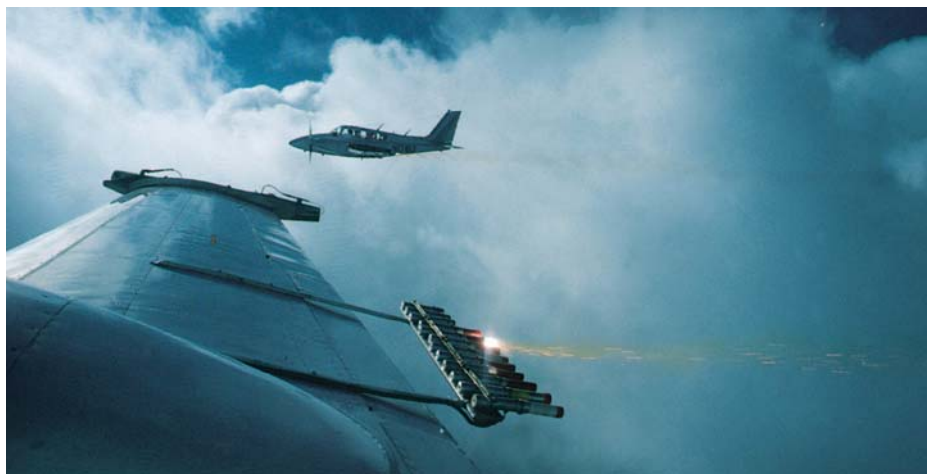
Figure 21.20 Cloud seeding using AgI particles.
