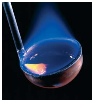
Sulfur burning in air to form \text{SO}_2 .
