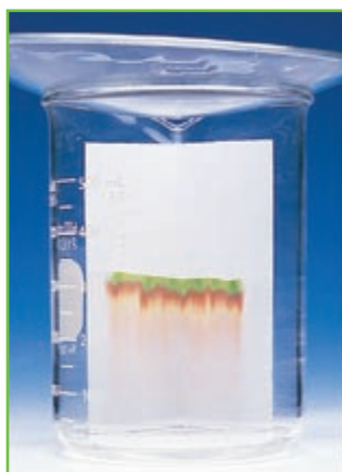
(b) The ink has separated and has risen up the paper. These actions are the result of specific properties of water molecules.
