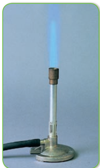
(a) In a Bunsen burner, methane combines with oxygen in the air to form carbon dioxide and water vapor.
