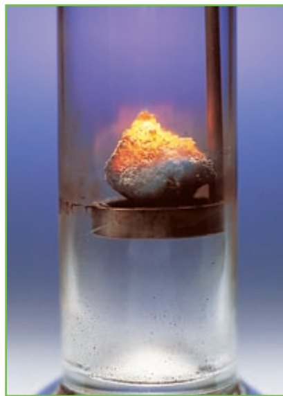
(a) Pure oxygen has five times the concentration of oxygen molecules compared to air, so the charcoal will burn more intensely.
