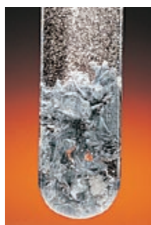
▲ Zinc reacts with dilute hydrochloric acid.
