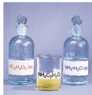
(d) The weak acid and weak base that form ammonium acetate are of comparable strength. A solution of ammonium acetate is essentially neutral.
