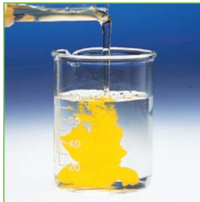
(b) When water solutions of ammonium sulfide and cadmium nitrate are combined, the yellow precipitate cadmium sulfide forms.
