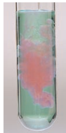
▲ Nickel (formation of a nickel dimethylglyoxime complex)
