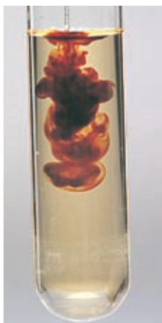
▲ Iron (formation of [\text{Fe}(\text{SCN})]^{2+} )
