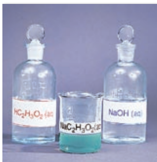
(b) The indicator shows the pH of the sodium acetate solution is basic. This was formed from a strong base and a weak acid.
