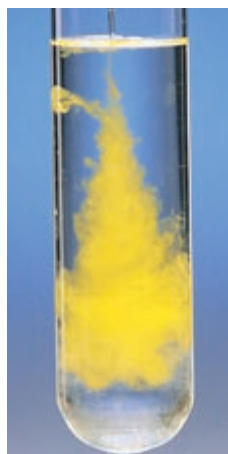
▲ Cadmium (formation of \text{CdS} )
