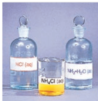
(c) The strong acid and weak base combination in ammonium chloride produces an acidic solution, as shown by the reddish tint of the indicator.
