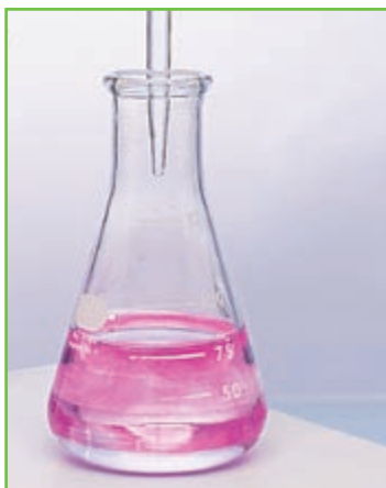
(a) Phenolphthalein turns pink at the end point.
