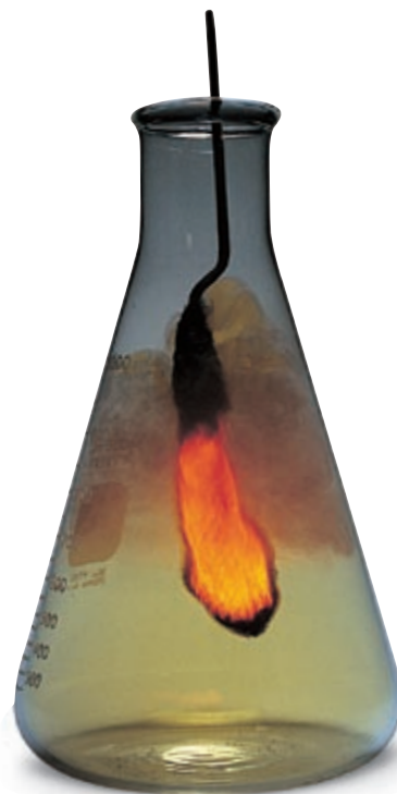
▲ Chlorine combines readily with iron wool, which ignites in chlorine gas to form \text{FeCl}_3 .
