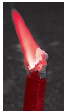
▶ A flare is made up of billions of reacting magnesium particles.
