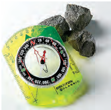
Magnetite is a magnetic ore containing \text{Fe}_3\text{O}_4 . Note that the compass needle points toward the ore.
