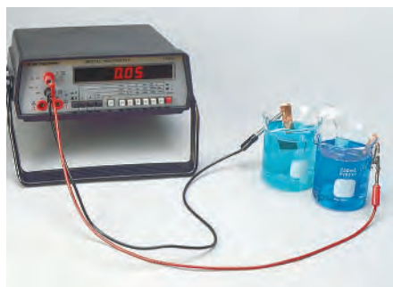
A concentration cell with 1.0 \text{ M Cu}^{2+} on the right and 0.010 \text{ M Cu}^{2+} on the left.
