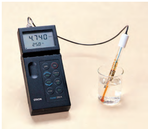
A digital pH meter shows the pH of the buffered solution to be 4.740.
