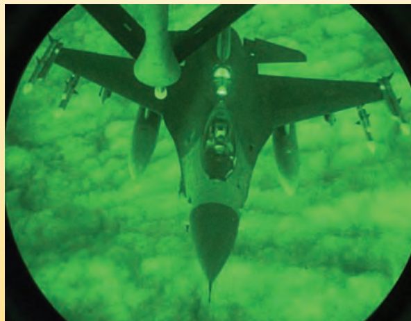
A night vision photo of the midair refueling of a U.S. Air Force plane.
