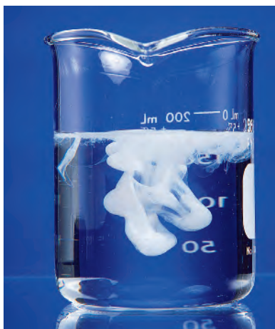
Figure 4.16 Precipitation of silver chloride by mixing solutions of silver nitrate and potassium chloride. The \text{K}^+ and \text{NO}_3^- ions remain in solution.
