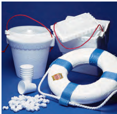
Blowing agents—such as hydrazine, which forms nitrogen gas on decomposition—are used to produce porous plastics like these polystyrene products.
