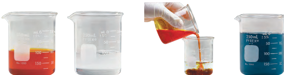
When potassium dichromate reacts with ethanol, a blue-violet solution containing \text{Cr}^{3+} is formed.
