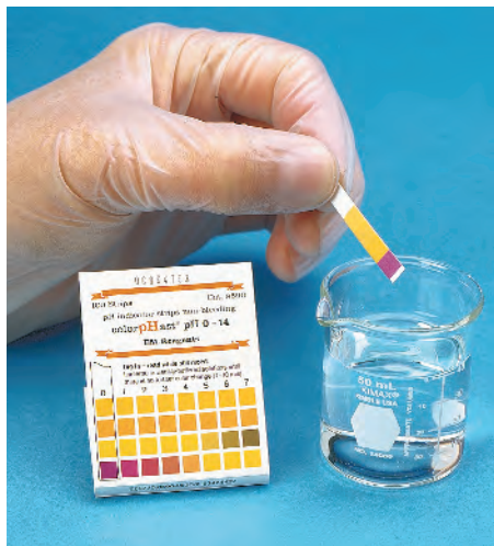
Universal indicator paper can be used to estimate the pH of a solution.
