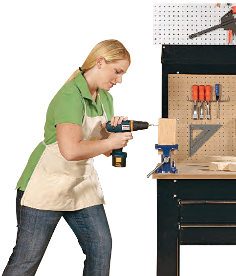
Using a battery-powered drill to insert a screw.
