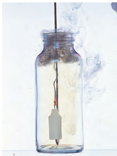
A candle burning in an atmosphere of \text{Cl}_2(g) . The exothermic reaction, which involves breaking C—C and C—H bonds in the wax and forming C—Cl bonds in their places, produces enough heat to make the gases in the region incandescent (a flame results).
