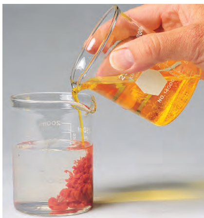
A potassium chromate solution being added to aqueous silver nitrate, forming silver chromate.
