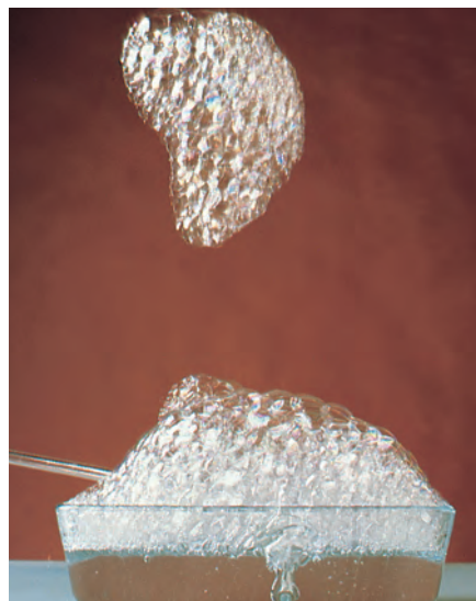
(left) Hydrogen gas being used to blow soap bubbles. (right) As the bubbles float upward, they are lighted by using a candle on a long stick. The orange flame results from the heat of the reaction between hydrogen and oxygen, which excites sodium atoms in the soap bubbles.
