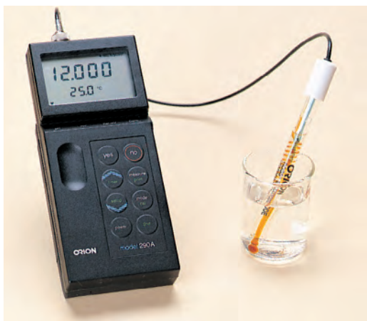
(top) Pure water at pH 7.000. (bottom) When 0.01 mol NaOH is added to 1.0 L pure water, the pH jumps to 12.000.
