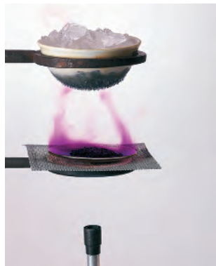
Figure 10.43 Iodine being heated, causing it to sublime, forming crystals of I_2(s) on the bottom of an evaporating dish cooled by ice.
