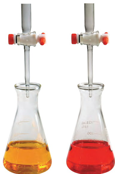
Methyl orange indicator is yellow in basic solution and red in acidic solution.
