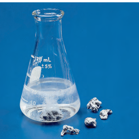
The reaction of zinc with hydrochloric acid to produce bubbles of hydrogen gas.
