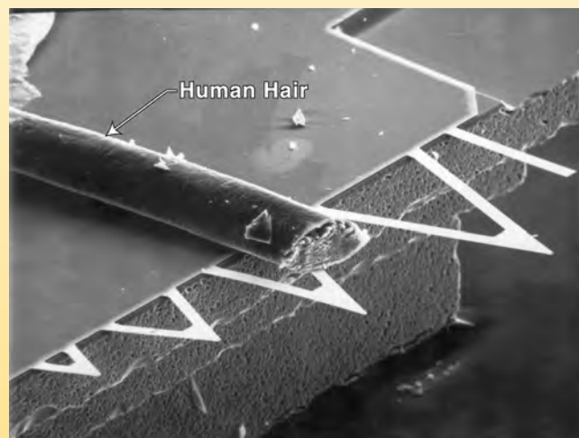
When explosive compounds bind to these V-shaped cantilevers, the microscopic structures, which are about the width of a hair, bend and produce a signal.
